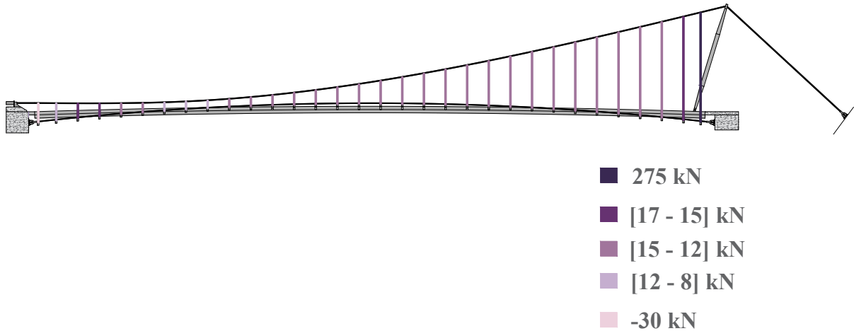
Figure 5.15: Tension distribution in the hangers with all hangers tuned identically.
