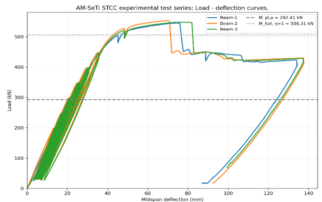
Figure 7 Midspan load-deflection curves: experimental curves vs. M_{pl,a} and M_{full, \eta=1} strain-controlled full composite
