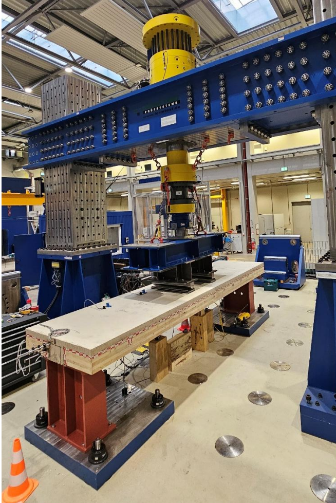
Figure 5 Specimen in testing frame
