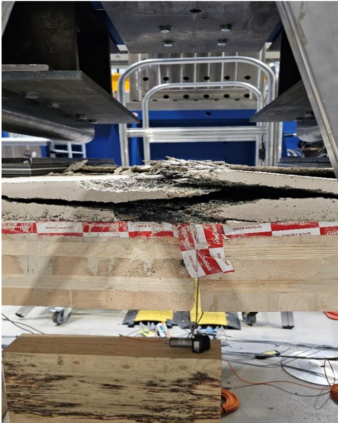
Figure 8 Failure mode: crushing of the concrete in the compression zone
