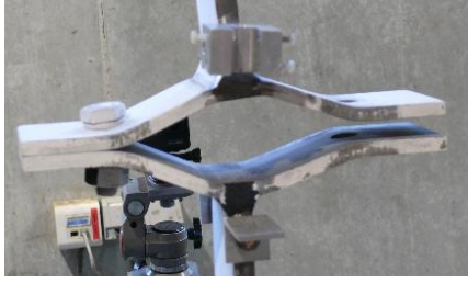
Figure 5 1R2C-10-690-BIS specimen at failure
