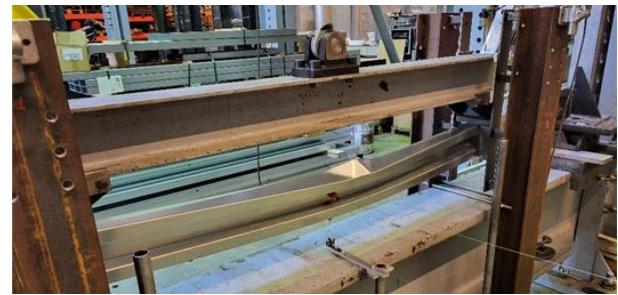
Figure 5 Indicative failure mode of local/global buckling interaction and yielding of the cross-section (Sp1a)
