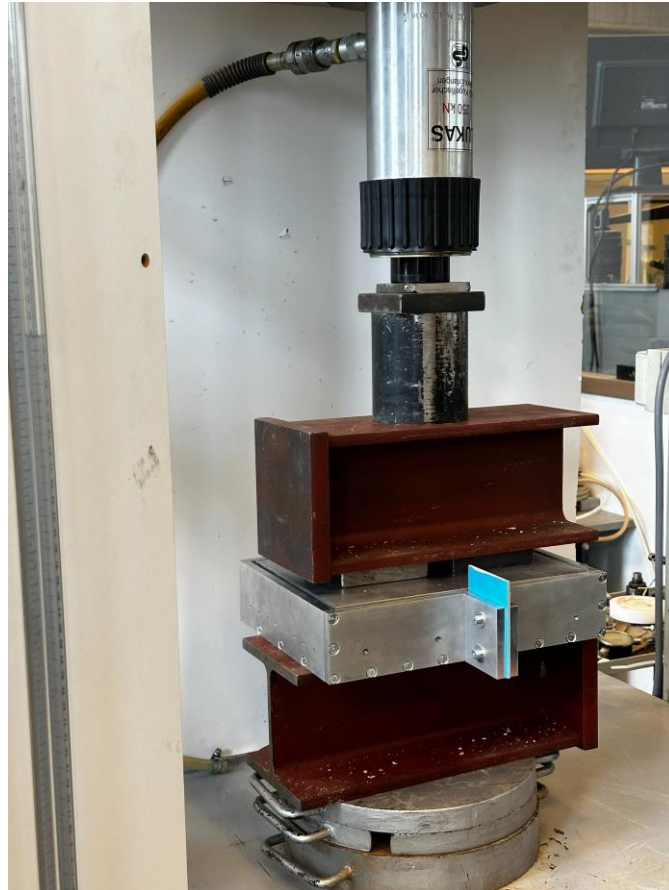
Fig. 5.5 Static compaction of the soil specimen inside the aluminium desiccation box using a hydraulic jack and a rigid steel plate to achieve the target dry density.
