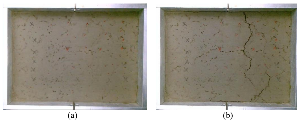
Fig. 5.17 Desiccation test results for S4 under unconstrained conditions: (a) specimen surface before crack initiation, (b) surface after cracking, (c) PIV-derived horizontal displacement field, and (d) PIV-derived horizontal linear strain field. Blue indicates extension and red indicates compression. Displacement and strain magnitudes are reported in calibrated physical units.
