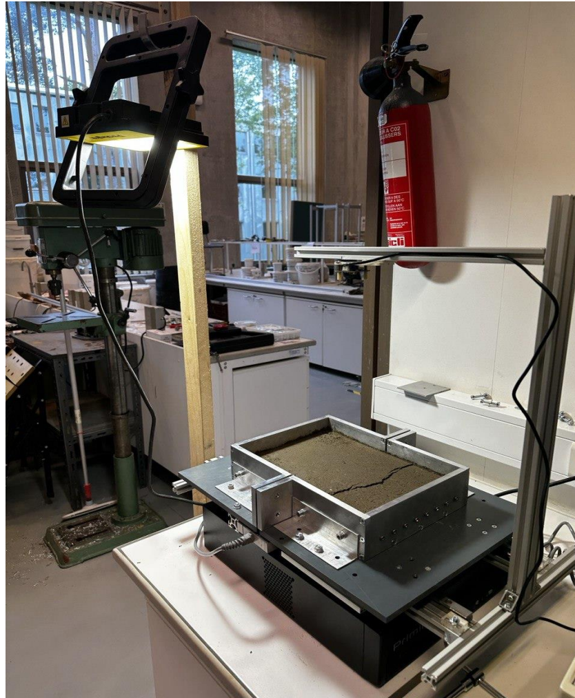
Fig. 5.7 Desiccation test setup showing the installed specimen, aluminum box, camera, and lighting system used for continuous monitoring and data acquisition.
