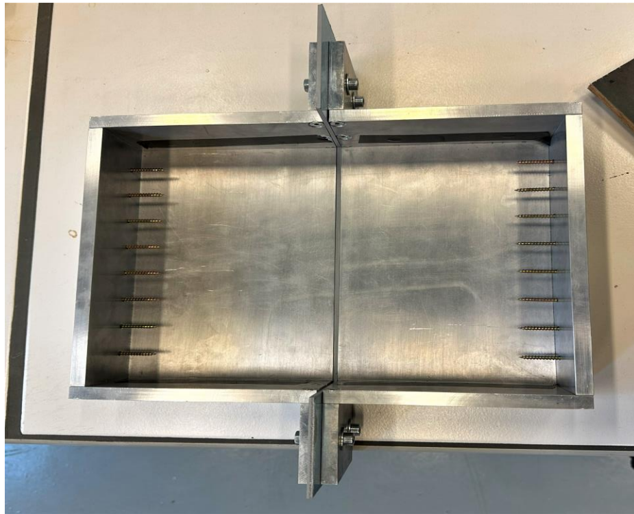
Fig. 5.1 Constrained desiccation box showing the end-wall screws used to anchor the soil.
