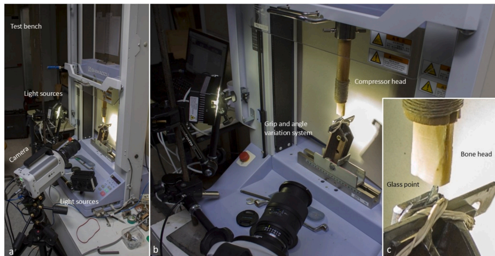
Fig. 2. Experimental setup for bench testing. (a) Overview of the test bench, light disposition and filming system, (b) view of the position of the piece before stress application, showing the grip and the angle variation system, and (c) close-up of the contact between the bone compressor and a glass specimen prior the stress application.
