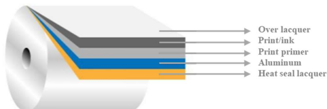
Figure 7. Structure of a multi-layer lidding foil.
