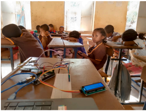
Fig. 3. In-situ measurements taken via Arduino recorder, Ambohimitsinjo (left) and Mangarivotra (right).
