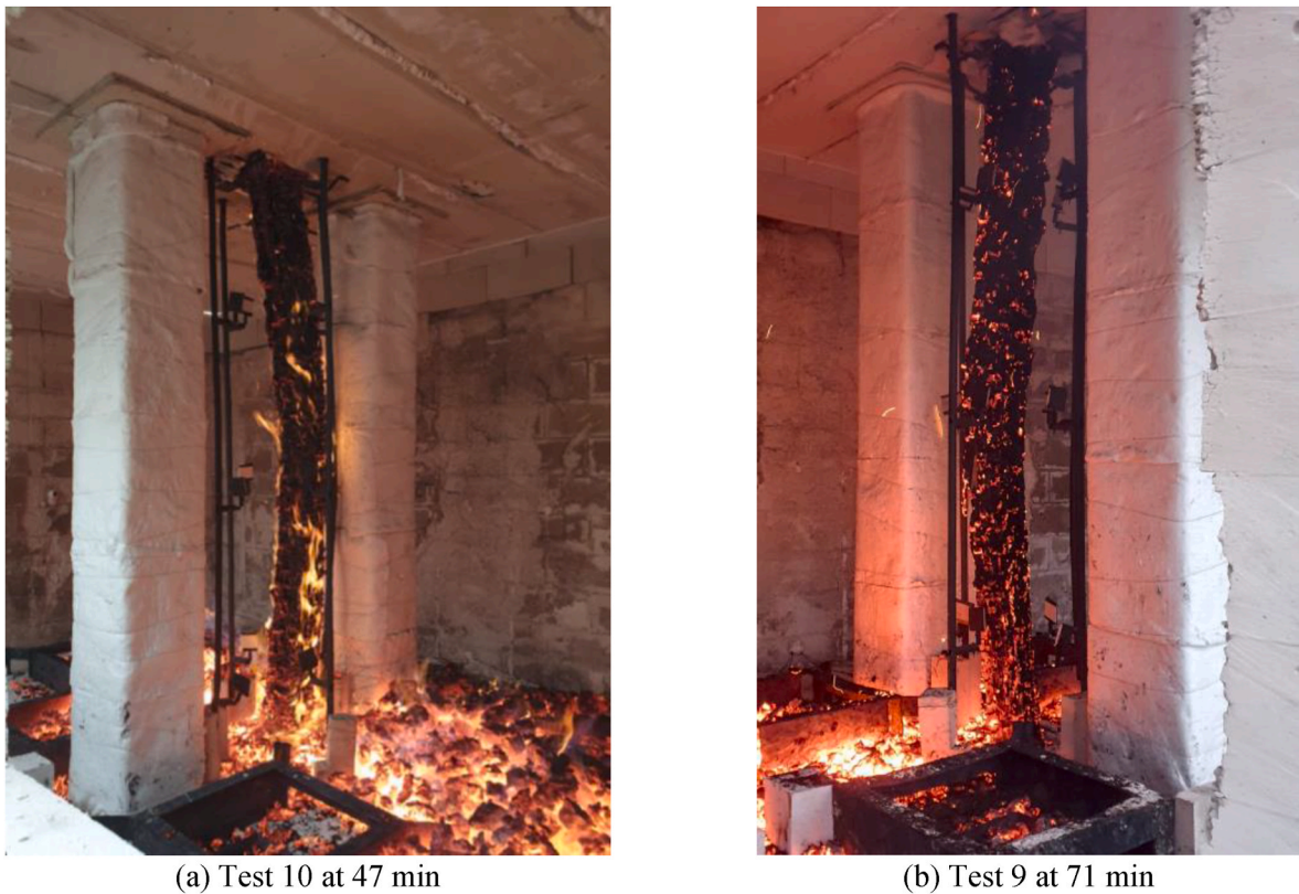
Fig. 5. Timber columns at the time of failure.
