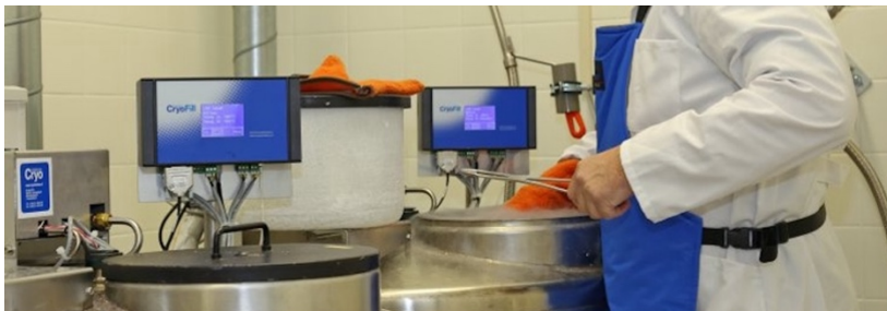
Figure 3.1 Photograph of nitrogen tanks for storing genetic material of animals. The technician holds a plier to place or remove semen straws. The screen displays the temperature and operation options. (Credits: Center for Genetic Resources, the Netherlands)
