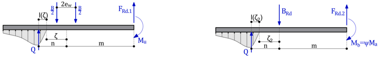
Fig. 10. Proposal for identifying the location of contact/prying forces [13]: a) Mode 1; b) Mode 2.
