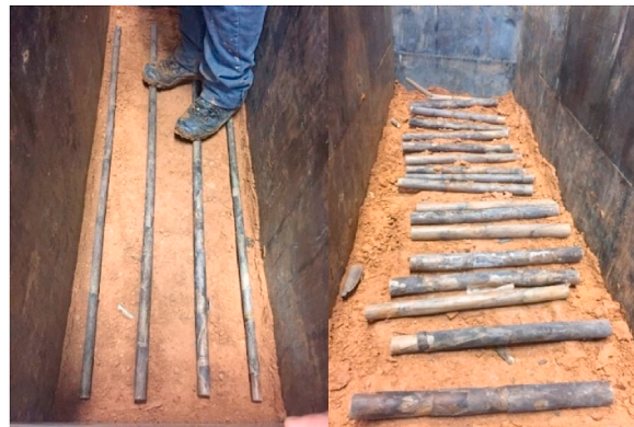
Fig. 3. Arundo donax left: Longitudinal sections and right: transversal sections.
