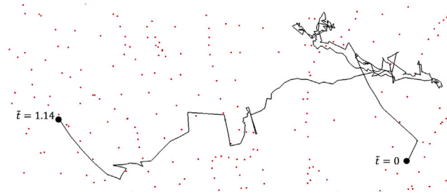
Fig. 10. Trajectory history of a representative SPH particle located in the projectile core using formulation 12 (moving least-squares based). Over \tilde{t} \in [0, 1.12] , the position exhibits pronounced unphysical oscillations, indicating numerical instability within the bulk.
