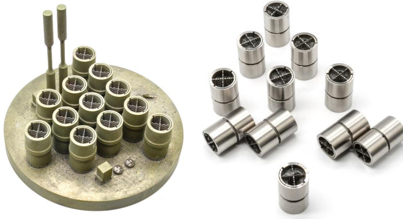
Figure 6: Manufactured Interlocked Lattice Flexure Pivots.
