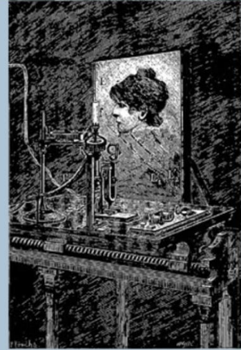
Telephot transmitter and receiver in Emile Desbeaux, Physique populaire , 1890
