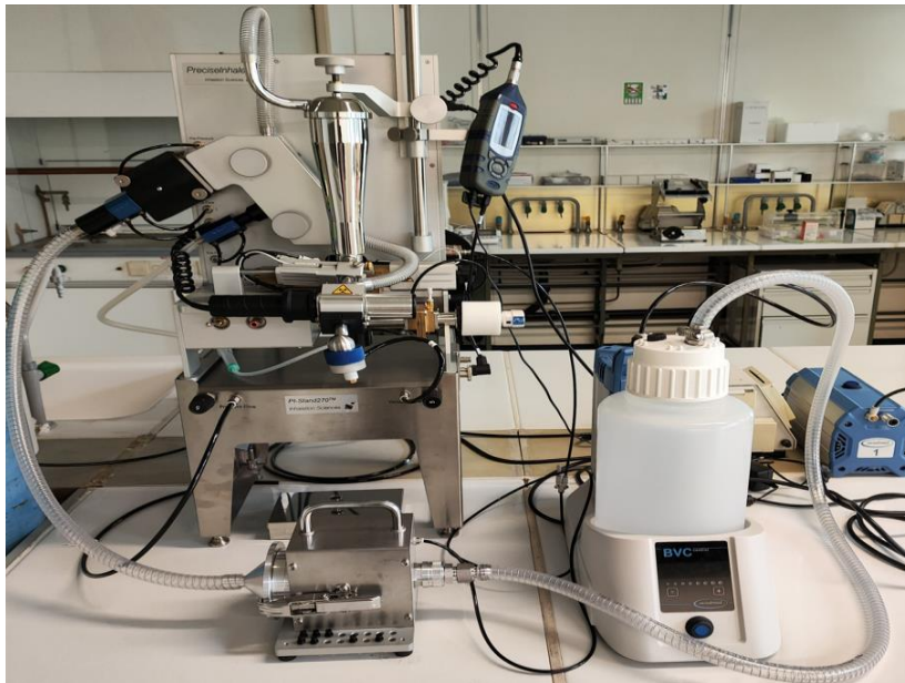
Figure 91: The PreciseInhale® system in the dry powder inhaler setup.
