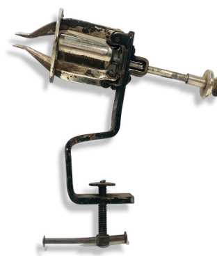
Figure 12, Mechanical device that stretches rubber rings to place over the pigeon's foot.
