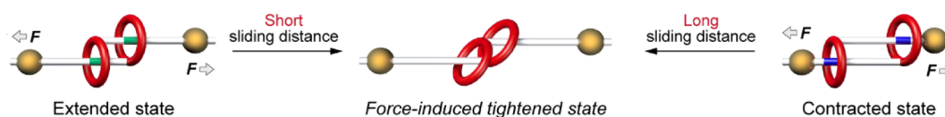
Figure 30. Schematic drawing of two bistable [c2]daisy chains each in a defined state (extended or contracted) used to prepare polymer networks. Adapted from ref. 163 with permission from the American Chemical Society, copyright 2023.
