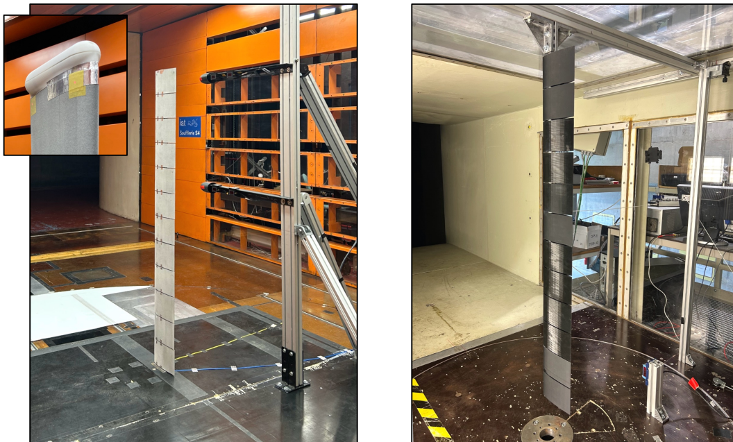
Figure 2: Experimental wind tunnel set-ups for the two wings: Wing 1 (left) and Wing 2 (right).
