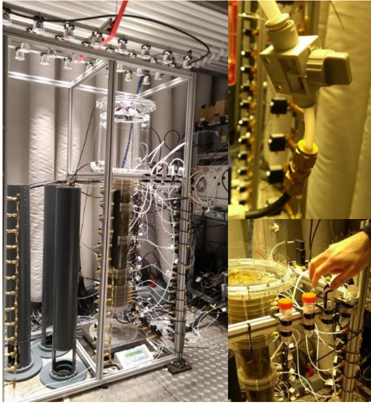
Fig. 20 Soil column during the water stable isotopes labelling, 7/12/2021. On the left, the acrylic soil column with the aboveground chamber without plants and the system for water stable isotopic measurements online is connected. On the top right, the manual valve to inject water in the soil dripping tubings. On the bottom right the labelled water to be injected
