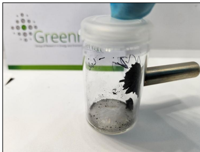
Figure 8 : Photograph of the powder being attracted to a hand-held magnet, showing the ferromagnetic character of the as-synthesized powder ( \text{Fe}(\text{OH})_3\text{-FeSi} particles).
