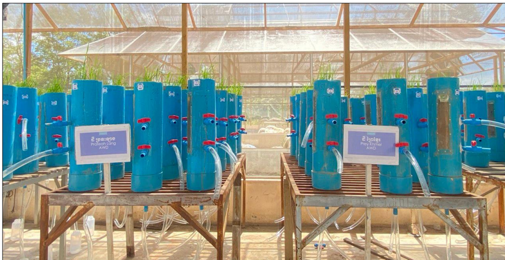
Figure 2-6: Soil column sampling: undisturbed condition
