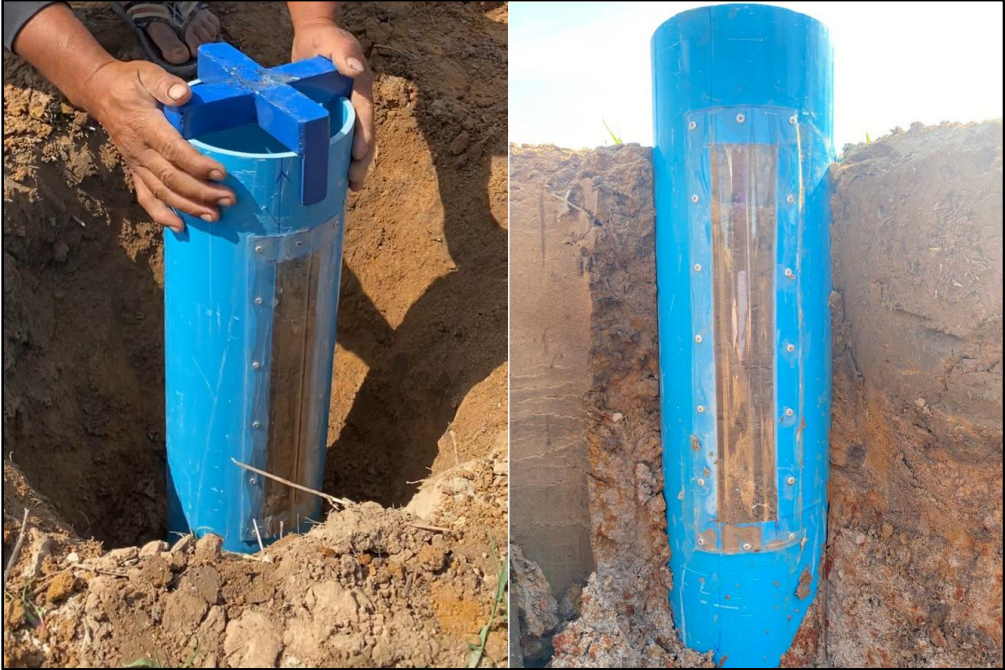
Figure 2-5: Soil column sampling: undisturbed condition
