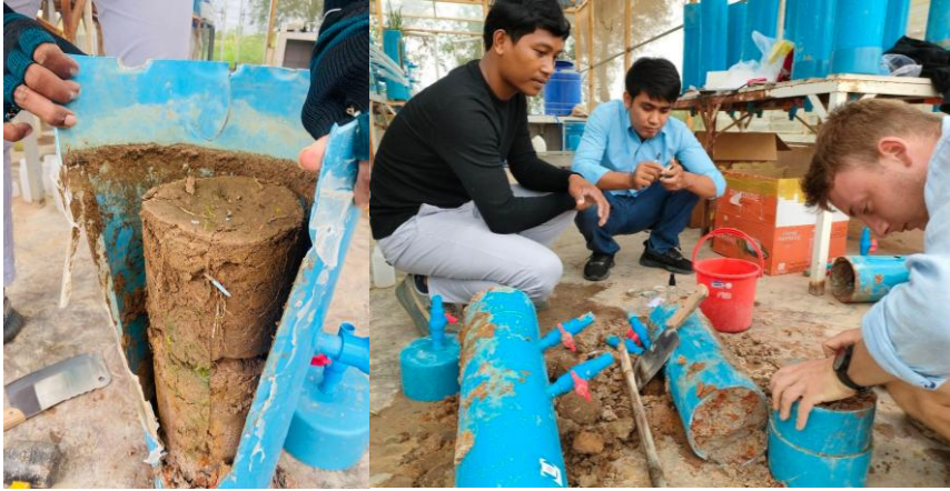
Annex 3: The activity involves breaking the soil column to collect samples of both roots and soil
