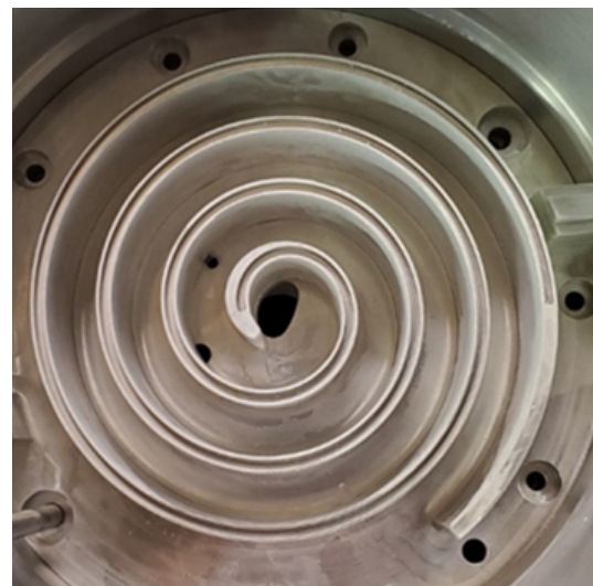
Figure B.6: Fixed scroll of the lab-scale prototype.
