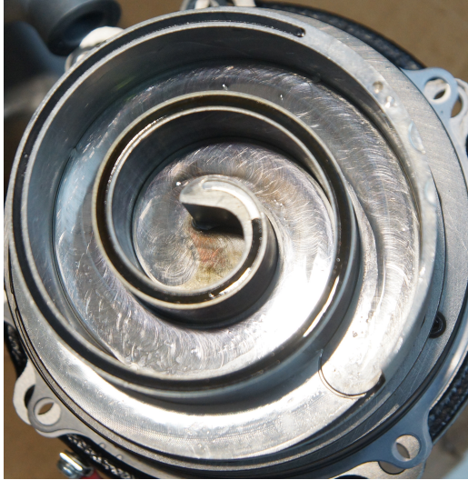
Figure 3.5: Orbiting scroll of the retrofitted compressor.
