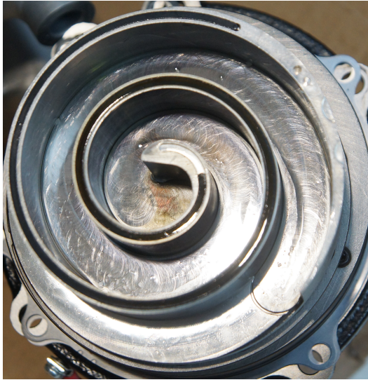
Figure B.3: Orbiting scroll of the retrofitted compressor.
