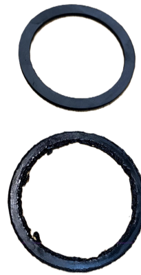
Figure B.8: Picture of the new sealing joint at the top and worn sealing joints at the bottom.
