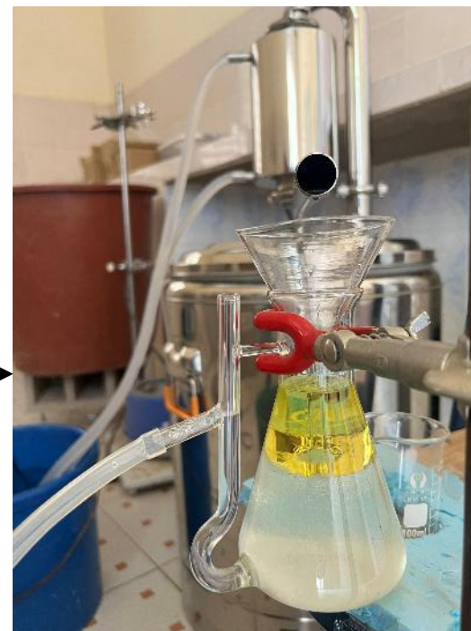
EO extracted by steam distillation using 2 kg of dry matter, 2 hours, n=3
