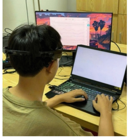
Fig. 1. Experimental protocol setup. Left: the Emotiv EPOC X headset used for EEG signal acquisition. Right: experimental setup where a participant wears the headset while performing a computer-based attention task.
