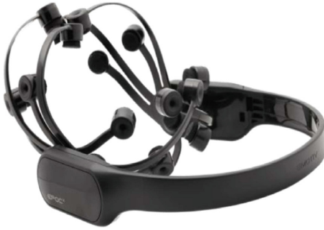
Fig. 1. Experimental protocol setup. Left: the Emotiv EPOC X headset used for EEG signal acquisition. Right: experimental setup where a participant wears the headset while performing a computer-based attention task.
