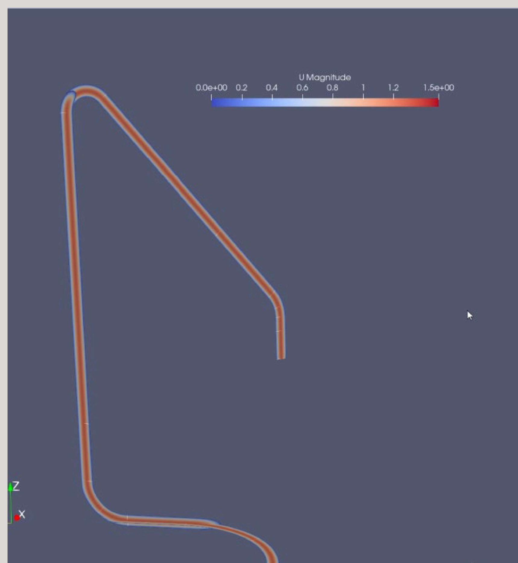
Fig. 3. Openfoam simulation to predict mortar flow behavior based on yield stress and viscosity of a 3D printable mixture
