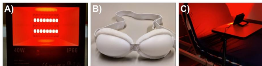
Figure 23. Equipment and Setup. A) Left – Flood Light: 40W total power, approximately 1000 lumens in each individual color setting (red and green). B) Center – Custom made Ganzfeld goggles: Created using plastic, transparent material cut at a curve such that placement over the eye orbits would create a homogenized visual field. The orbits of the plastic were padded using white foam for comfort and connected with adjustable inter-ocular distance bands and an adjustable headband. C) Right – Medical Bed: In a typical MMGF session with red light and white noise, a prospective participant would lie on the reclined medical bed with the goggles fitted comfortably and properly (i.e., the cover the eye orbits and prevent light leakage). The lamp is placed such that it is approximately 40cm from the eyes. The volume of the white noise is adjusted per participant to what they find comfortable.
