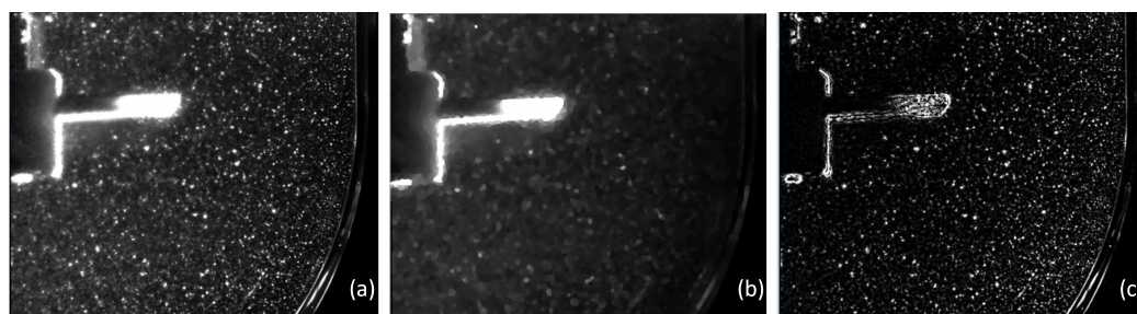
Figure 4. Instantaneous PIV images from solids camera at \alpha_p = 0.5 v%: (a) Raw image. (b) Generated background filter. (c) Treated image. The impeller is evidently masked prior to obtaining vector maps.
