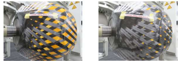
Figure 2: Filament winding on the soccer-ball mandrel
