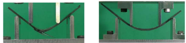
Figure 3: 4-points bending on coupons in longitudinal (left) and circumferential (right) directions, extracted from the dome
