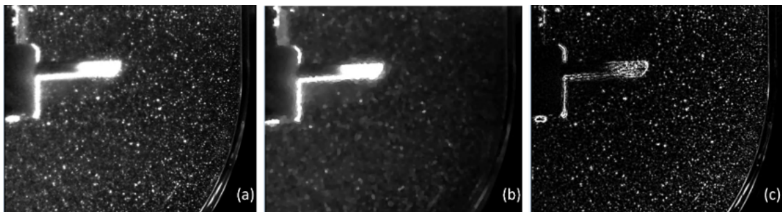
Figure 3.4: Instantaneous PIV images from solids camera at \alpha_p = 0.5 v%: (a) Raw image. (b) Generated background filter. (c) Treated image. The impeller is evidently masked prior to obtaining vector maps.
