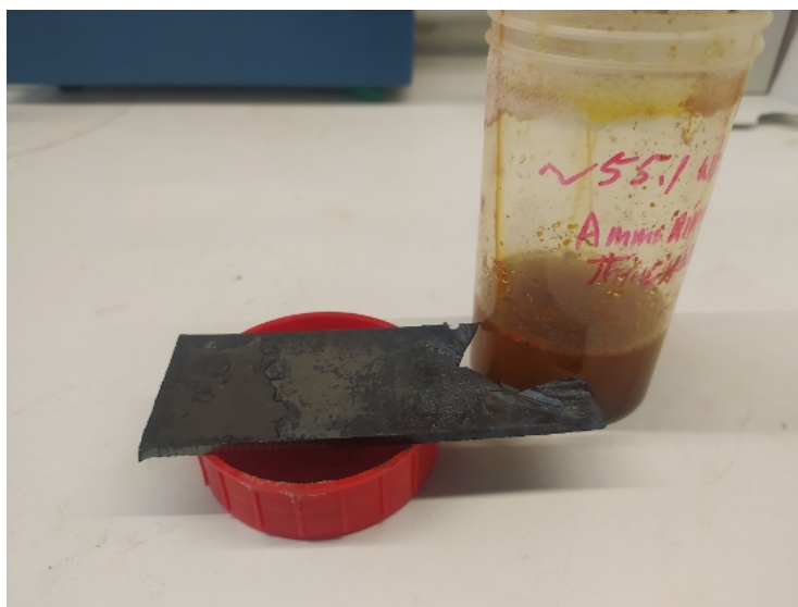
Figure A.1.1: Corrosion effect of \text{NH}_4\text{SCN} in contact with plain steel. Duration: 3 - 4 days.
