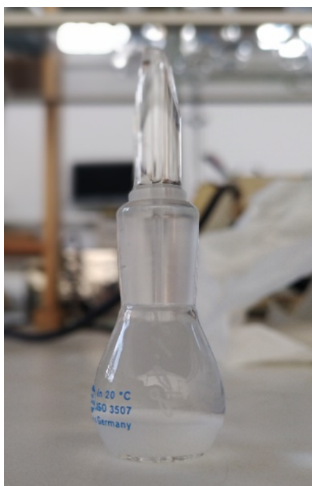
Figure A.1.3: 5-mL volumetric Pycnometer filled with PMMA particles and water
