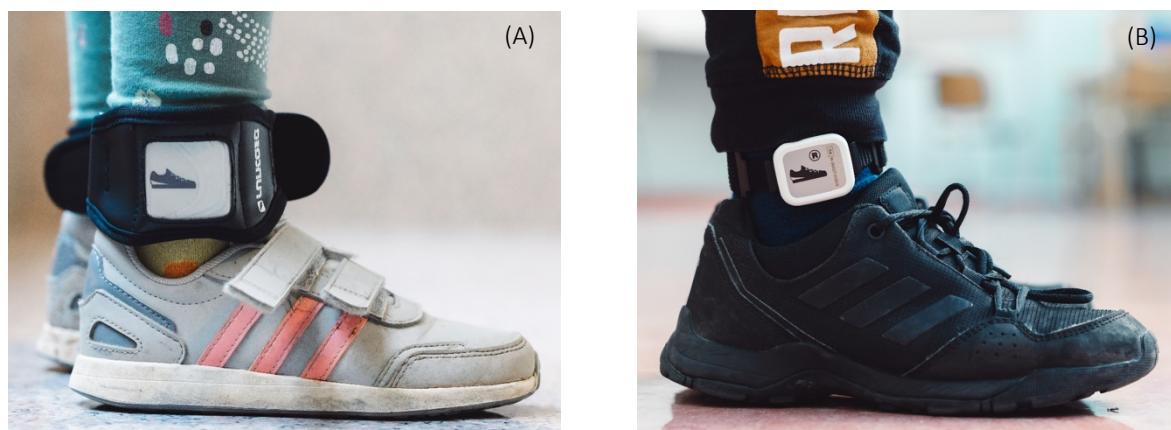
Figure 5. Images of the ActiMyo® (A) and Syde® (B) devices.
