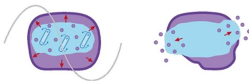
Figure 4. Extraction process promoted by MW irradiation
