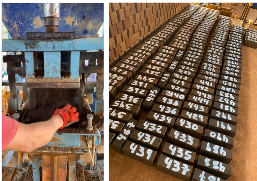
Fig. 2. Manufacture of compressed earth blocks.
