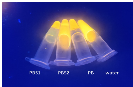
Figure 5.6. Picture of the redispersed QDs, under 365 nm irradiation, in the 3 phosphate buffers and water for control.
