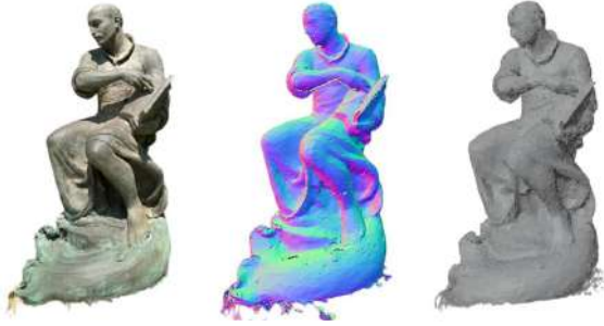
Figure 10. Object extraction. Additional visual examples demonstrating the object extraction capabilities of MeshSplatting. From left to right: generated RGB image of the object, estimated surface normals, and resulting mesh representation.
