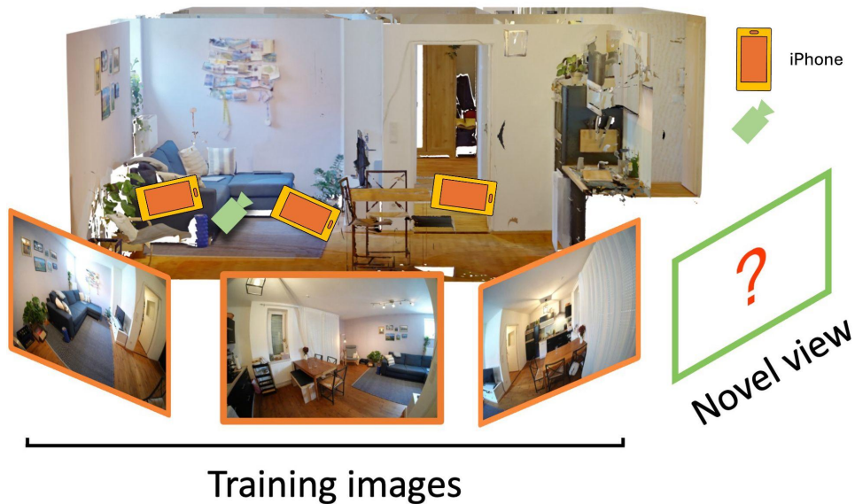
Figure 2.1.: Overview of novel view synthesis. The goal is to render the scene from novel camera poses that were not observed during training, while preserving the appearance and structure consistent with the input views. The image is taken from [10].
