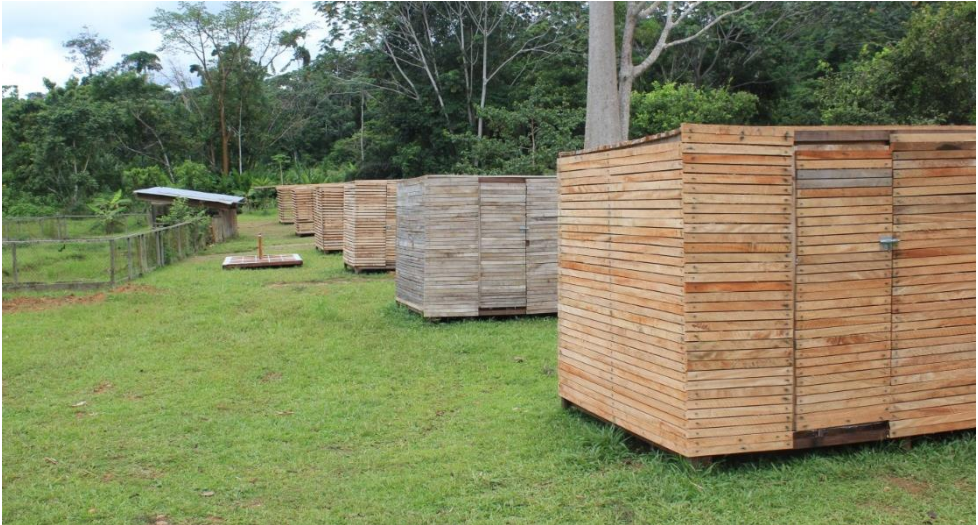
Figure 15 : Experimental setup including six shade houses receiving, from front to back, 4%, 1%, 10%, 25%, 40%, and 60% of Relative Irradiance (RI), and a platform (left) receiving 100% RI. The structures were built in 2019 for a similar experiment on Cylicodiscus gabunensis (Okan) (Ndonda Makemba, 2023), and were inspired by the protocol of Agyeman et al. (1999).
