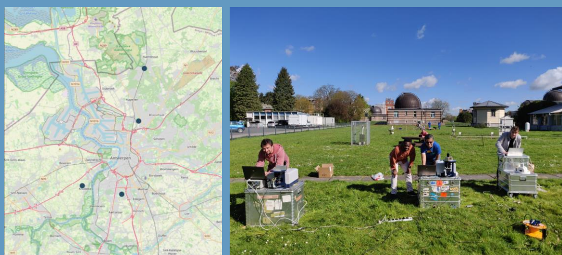
Figure 1. Left: FTIR instrument locations around Antwerp during the campaign. Right: Intercomparison of four mobile instruments at BIRA-IASB, Uccle, before the campaign.
