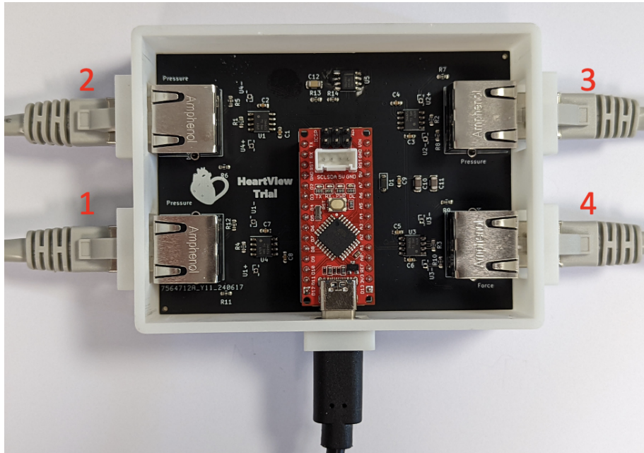
Figure 7.10: DAQ unit with port numbers labelled. Ports 1 - 3 are for pressure sensor inputs, and port 4 is for the load cell input.
