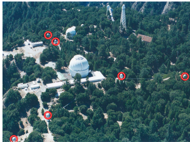
Figure: The CHARA interferometer composed of six 1m telescopes at Mount Wilson Observatory (California, USA). © The Observatories of the Carnegie Institution.
