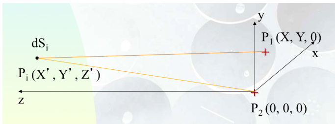
Figure: Positions of the two elements P_1 and P_2 of the interferometer and of the infinitesimal element P_i of the source assuming that the distance Z' \gg |X'|, |Y'|, |X| or |Y| .
