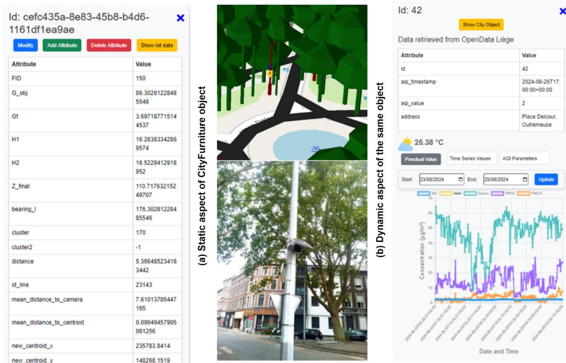
Figure 4.9. The CityThings concept applied to a sensor in the study area: (a) Static attributes from the modeling process, (b) dynamic attributes from the STA DB.
