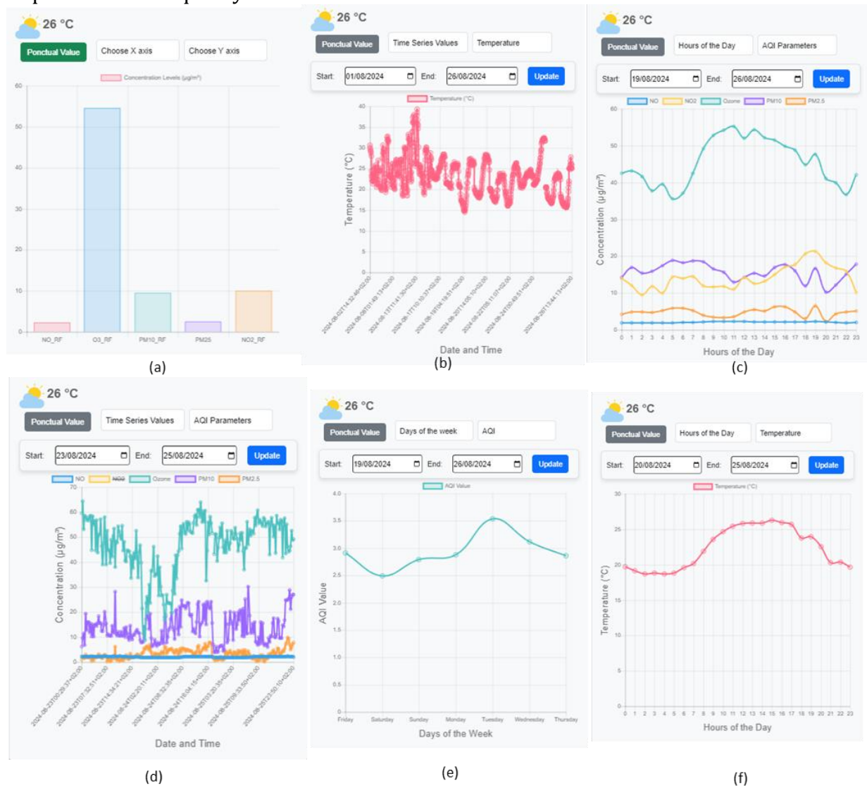
Figure 4.20. Time series analysis of air quality: (a) Concentrations of each pollutant at time t; (b) Temperature variations from 08/01 to 08/26; (c) Average hourly concentrations calculated between 08/19 – 08/26; (d) Concentration variations between 08/23 and 08/25; (e) Average daily concentrations calculated between 08/19 – 08/26; (f) Average hourly temperatures calculated between 08/20 – 08/25.
