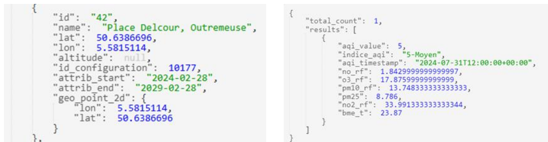
Figure 4.2. Retrieved API responses for sensor ID = 42: sensor metadata and location (left) and air quality observations (right).
