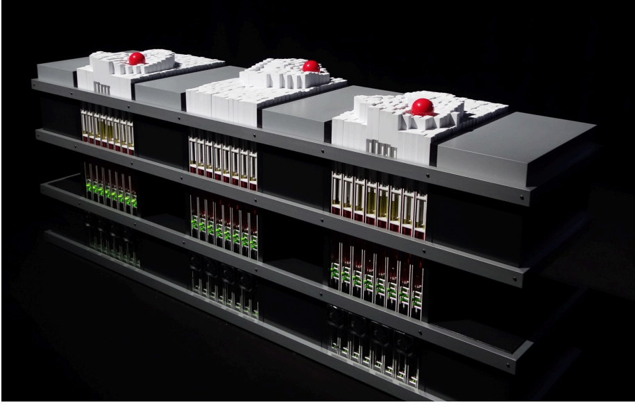
Figure 8.3: The MIT TRANSFORM table The system consists of a dense array of vertically actuated pins whose heights can be individually controlled to render dynamic three-dimensional shapes in real time [119]. Adapting a similar concept to an immersed platform would enable programmable spatiotemporal control of the liquid interface curvature. © 2012 Tangible Media Group / MIT Media Lab.
