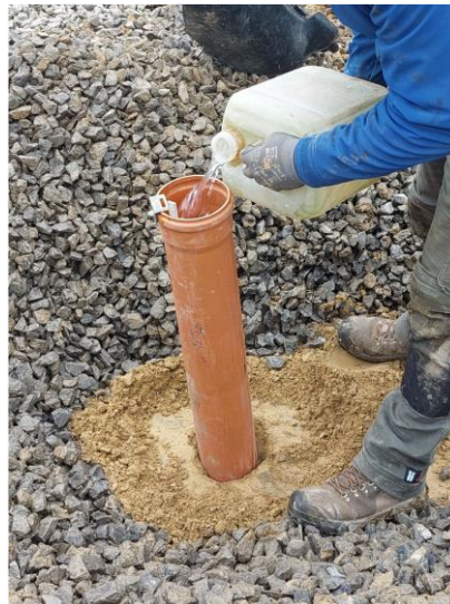
Figure D1. Porchet method illustrated in a shallow well within loess sediments.
