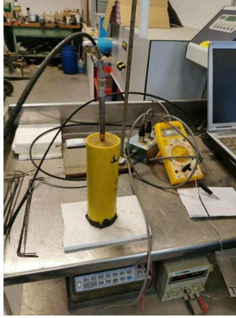
Figure D4. Needle probe measurement method of thermal conductivity on saturated loess sample.
