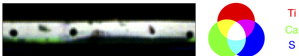
Figure A5. MA-XRF of the exposed ground in a tacking margin showing the presence of titanium (Ti), calcium (Ca) and Sulfur (S), showing the presence of \text{TiO}_2 and \text{CaSO}_4 .
