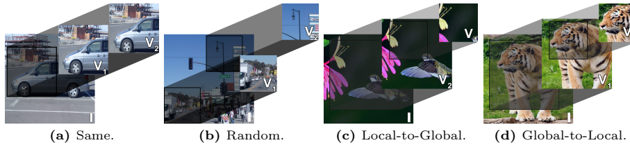
Fig. 2: Illustration of our four cropping strategies. For a given input image I , we generate an unmasked view V_1 and a masked view V_2 following one of four different cropping strategies: (a) Same Views, where V_1 = V_2 ; (b) Random Views, where V_1 and V_2 are two independent random crops; (c) Local-to-Global, where V_1 is a random crop within V_2 , and (d) Global-to-Local, where V_2 is a random crop within V_1 .
