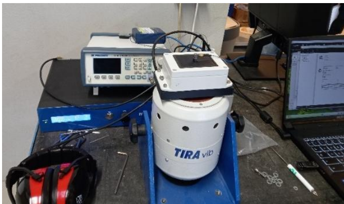
Fig. 3. Laboratory validation of the instrumentation using a vibration shaker.
