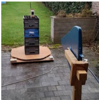
Fig. 6. Left: Characterization of the radiation pattern of the antenna with the device placed vertically on a rotating platform. Right: Radiation pattern of the meander-shaped PCB antenna measured in continuous-wave mode (15 dBm) for a vertically oriented device rotating around a vertical axis. The red and blue curves correspond to horizontal and vertical polarizations, respectively.
