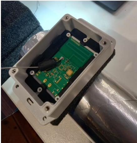
Fig. 5. Study of the stay cable's impact on antenna tuning. The meander-shaped PCB antenna is visible on the right side of the PCB.
