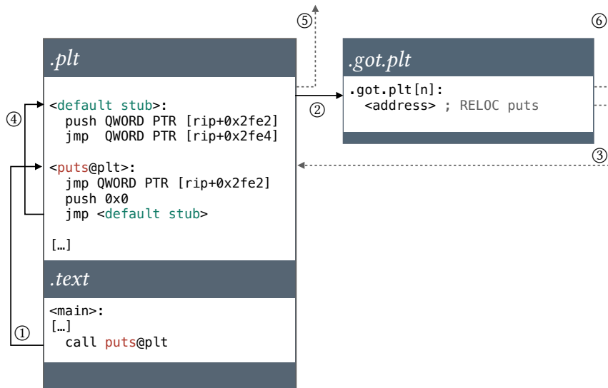
Figure 2.3: Using the PLT and GOT to call external functions. The dynamic linker resolves the address of puts the first time it is called.
