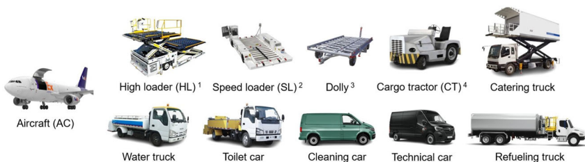
1 Lift between ground and aircraft door, 2 Transfer vehicle between HL and dollies, 3 Non-motorized trolleys, 4 Towing vehicle for dollies
