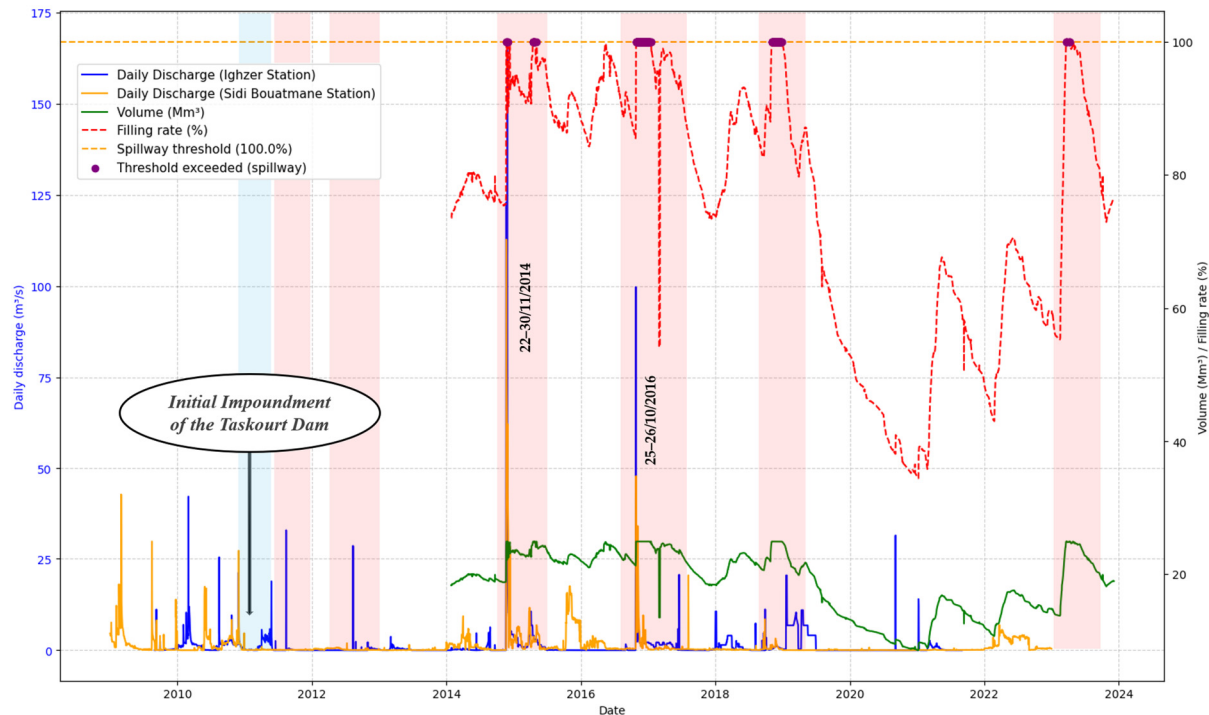
Figure 7. Daily variation in discharge and filling status of the Taskourt Dam (blue band: initial impoundment; red bands: recorded events).
