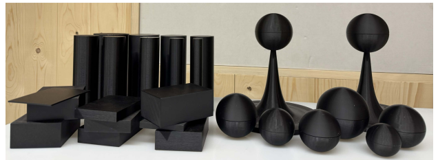
Fig. 4. The Shadow Dexterous Hand is used to evaluate the robustness of the proposed approach on 27 3D-printed primitive-shaped objects spanning the typical range of daily-life object dimensions.
