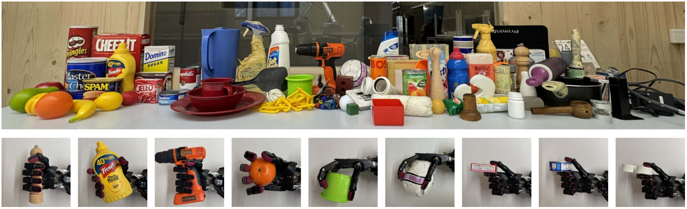
Fig. 8. Shape primitives are expressive enough to cover a broad range of household objects. The method achieves a success rate of 77% on the YCB subset and 82.5% on the full set of 80 objects. YCB objects appear on the left; additional everyday objects on the right.
