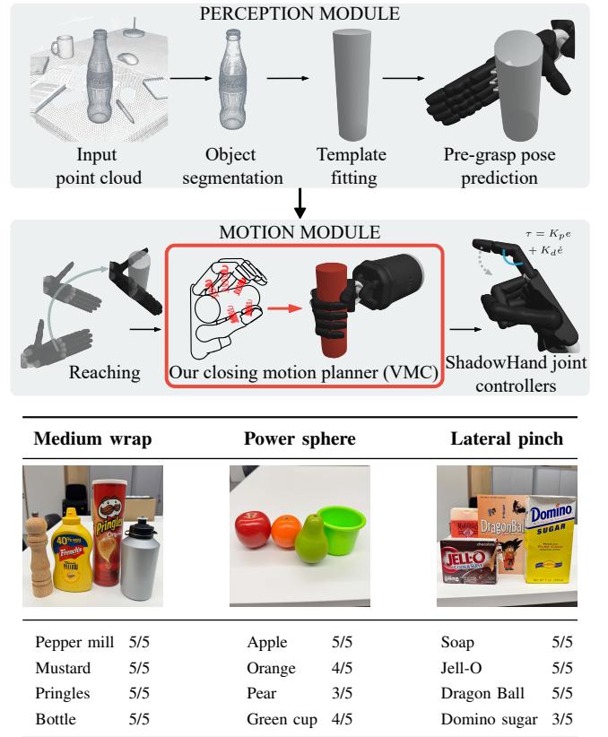
Fig. 8. Within an autonomous pipeline, the planner grasps 12 everyday objects in 54 of 60 trials (90 %). Top: pipeline modules, with our planner outlined in red. Bottom: successes over five trials per object, grouped by grasp type.
