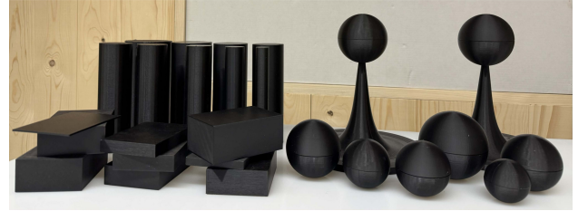
Fig. 4. Robustness tests use 27 3D-printed cylinders, spheres, and boxes (bottom), grasped by a Shadow Dexterous Hand on a UR10e arm (top).
